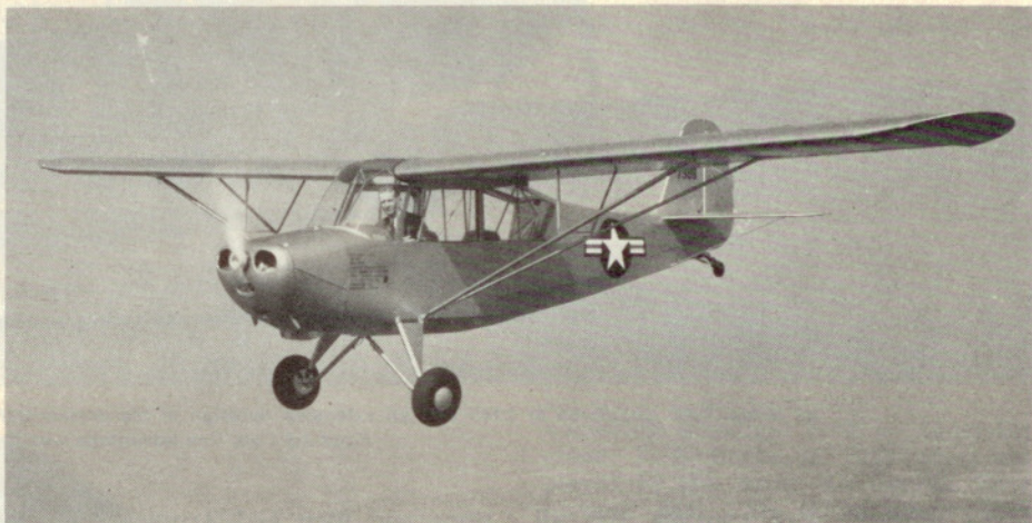
The Army gave its only postwar ultralight business to Aeronca for 85-hp L-16A versions of the Champion (shown) and 90-hp L-16Bs with dorsal fins.
