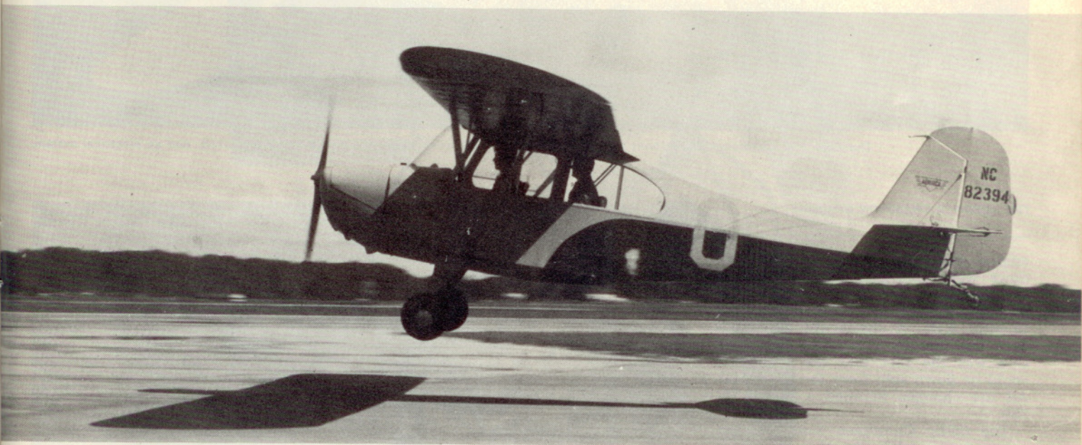
The Model 7-AC Champion of 1945 was an extensive redesign of the prewar Defender intended to compete more effectively with the Piper J-3 Cub. One advantage was that the Champ could be flown solo from the front seat.
