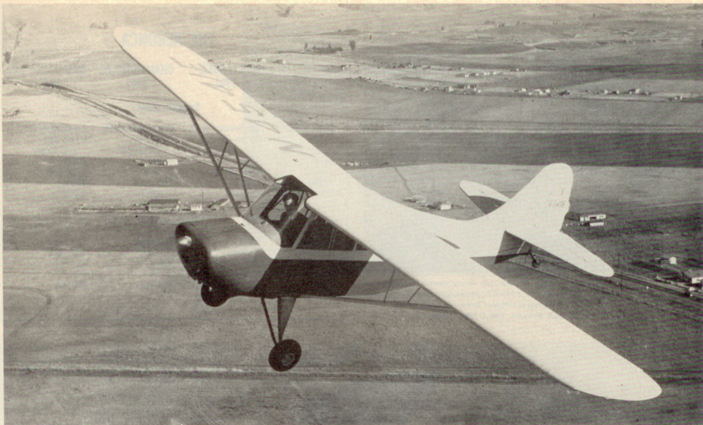
The final civil Champion model built by Aeronca was the 7-EC, with 90-hp, the dorsal fin of the L-16B, and an electrical system.
